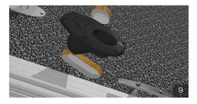
TEST THAT THE DECK RECEPTACLE DROPS NEATLY INTO THE OVAL SHAPE YOU'VE JUST CUT. If it is too tight to gently tap into place, then use a wood rasp or sandpaper to touch up the inside edge of the cut you've made until the deck receptacle fits. A fit that requires lightly tapping the deck receptacle into place is perfect.
